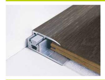
The patented MULTICLIP CLP 270 aluminum perimeter profile allows floor edge finishing without baseboards. A 5/8" (16mm) internal cavity allows 3/16" (5mm) of differential movement. This profile is also suitable along sliding door tracks and as entrance mat framing.
